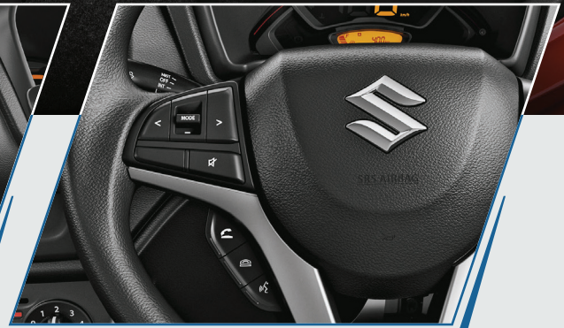
STEERING MOUNTED AUDIO AND VOICE CONTROL
